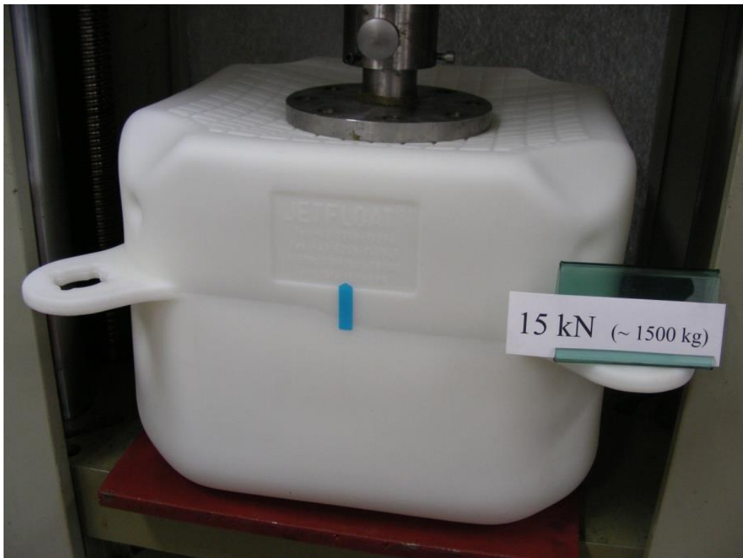
Picture 4: Load level 15 kN
