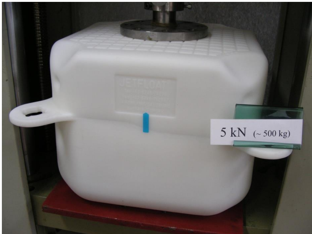
Picture 2: Load level 5 kN
