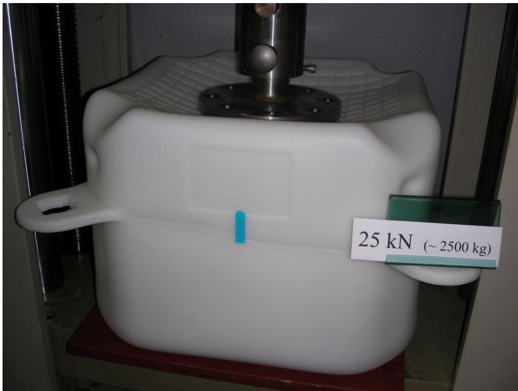
Picture 6: Load level 25 kN
