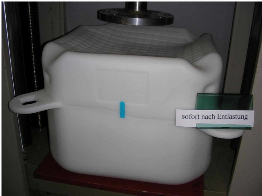
Picture 8: Condition immediately after release
